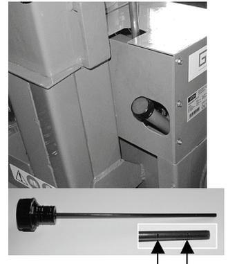
Now screw up the drain screw again. **Caution! No impurities can get in any circumstances in the hydraulic oil tank.** Now fill in the hydraulic oil tank and check whether there is a correct hydraulic oil level in the tank using a gauge. **Attention: Always fill the oil only when the splitting post is inserted!**
