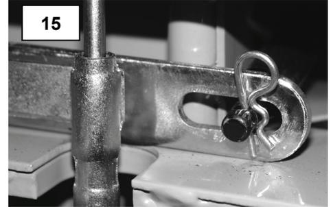
Now insert the safety pins included in the supply to the back of the bracket with operating arm as illustrated in (**pic. 15**).
