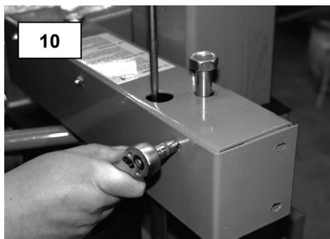
1. Unscrew the operating arm bracket (pic. 10)
